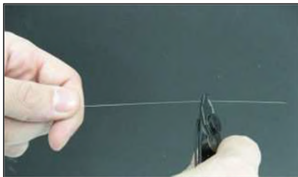
Figure 13 Stripping Fiber using a Miller Stripper
