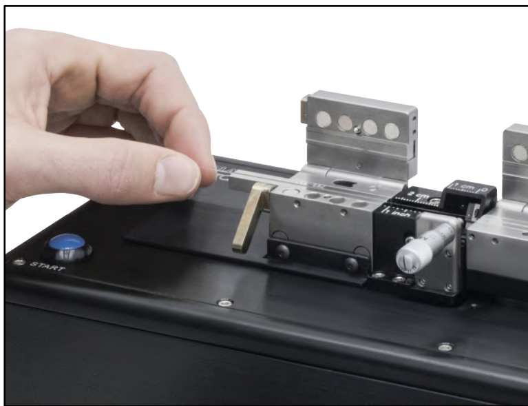
Figure 16 Removing a Cleaved Fiber from the Left Fiber Holding Block
