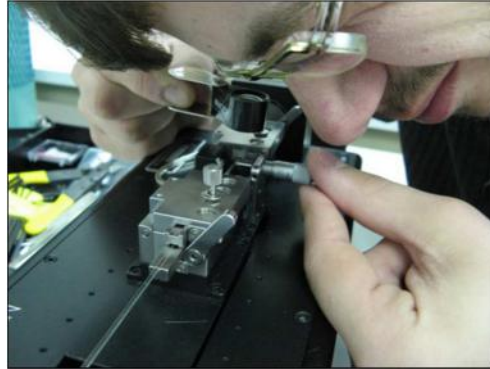
Figure 20 Using an Eye Loupe to Check that the Micrometer Backstop just Touches the Fiber
