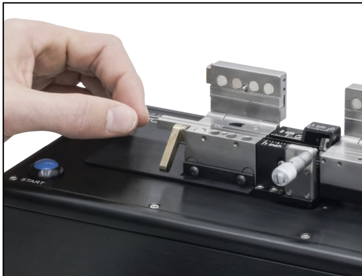
Figure 14 Positioning a Fiber in the Left-Hand FHB V-Groove
